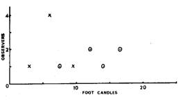
Number of observers against just adequate illumination level for neutral bock-ground. Crosses, illumination increasing. Circles, illumination decreasing.
