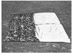
A shiny fabric (right) contrasts sharply with the grass background. The same fabric is shown on the left after being incised, or cut into with short curved knives. (Crown copyright.)
