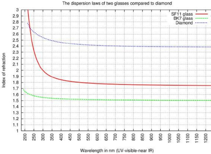
**Figure 1:** Comparison of three dispersion curves of transparent materials on the UV-visible-near IR interval. Two glasses, BK7 and SF11, are compared to diamond. It is obvious that all the indices have higher values in the UV region and consequently a higher power of refraction for that part of the spectrum.
