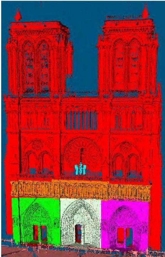
**Figure 15:** Results of the 3D scanning process obtained by the 2 GX and FX set of sensors. About 53 million of 3D points were acquired.
