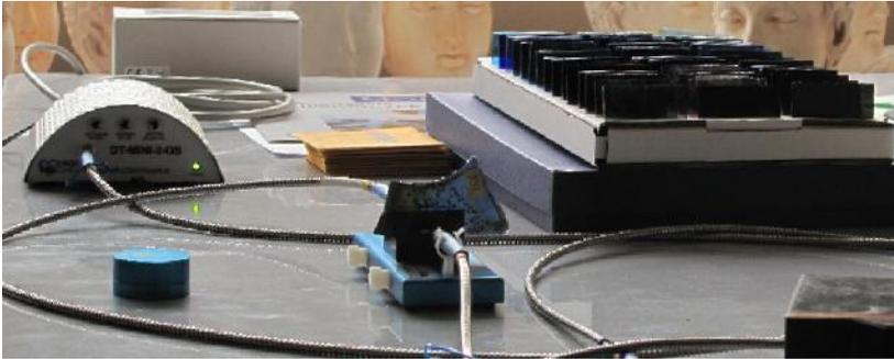
**Figure 4:** Spectrophotometric measurement of the transmitted light by a medieval glass sample. A set of medieval-like glasses are used for visual comparison with the authentic sample and to measure their optical constants by spectroscopic ellipsometry. That work is in progress for retrieving the most probable natural lighting in the abbey-church of Royaumont. Here is shown a sample in the measuring head (centre) on the bench with light source, fibre optics and standard samples (right).
