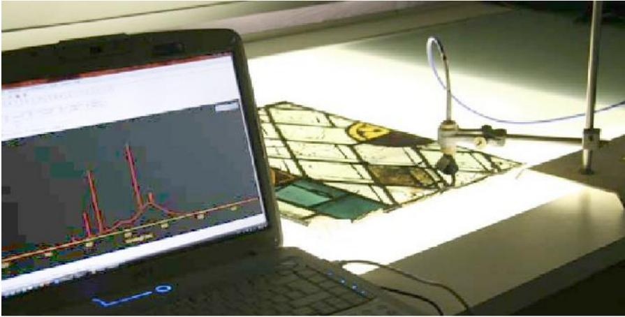
**Figure 6:** Spectrophotometric measurements of the transmitted light by a medieval stained glass window at LRMH (Laboratoire de Recherche des Monuments Historiques). We have also used several light sources.
